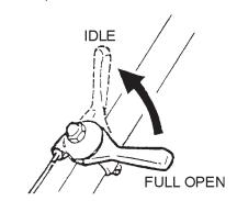
Figure 10. Throttle Lever (Idle)
